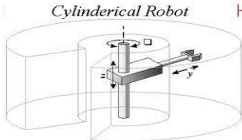
Fig 2: Cylindrical configuration [5]
